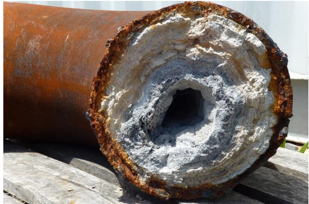
Extreme silica scaling of 450mm pipe at Ohaaki, NZ
