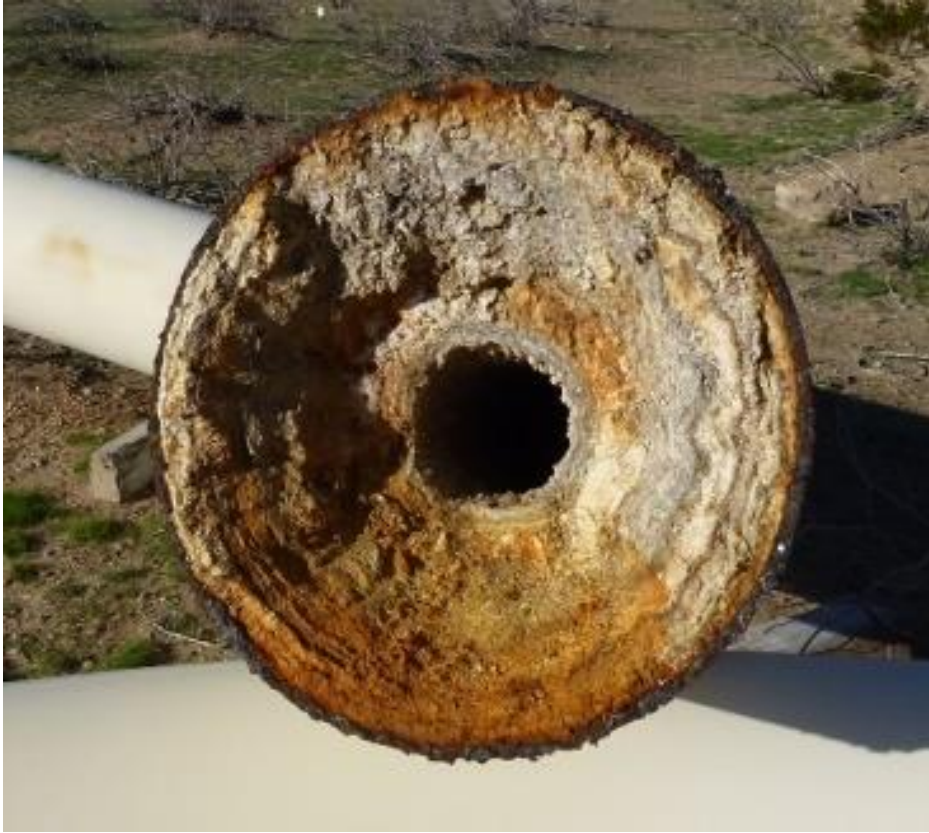
Silica scaling of 450mm reinjection pipe at Coso, California, USA
