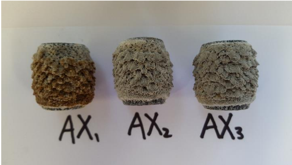
Inlet scaling coupons after 6 months
