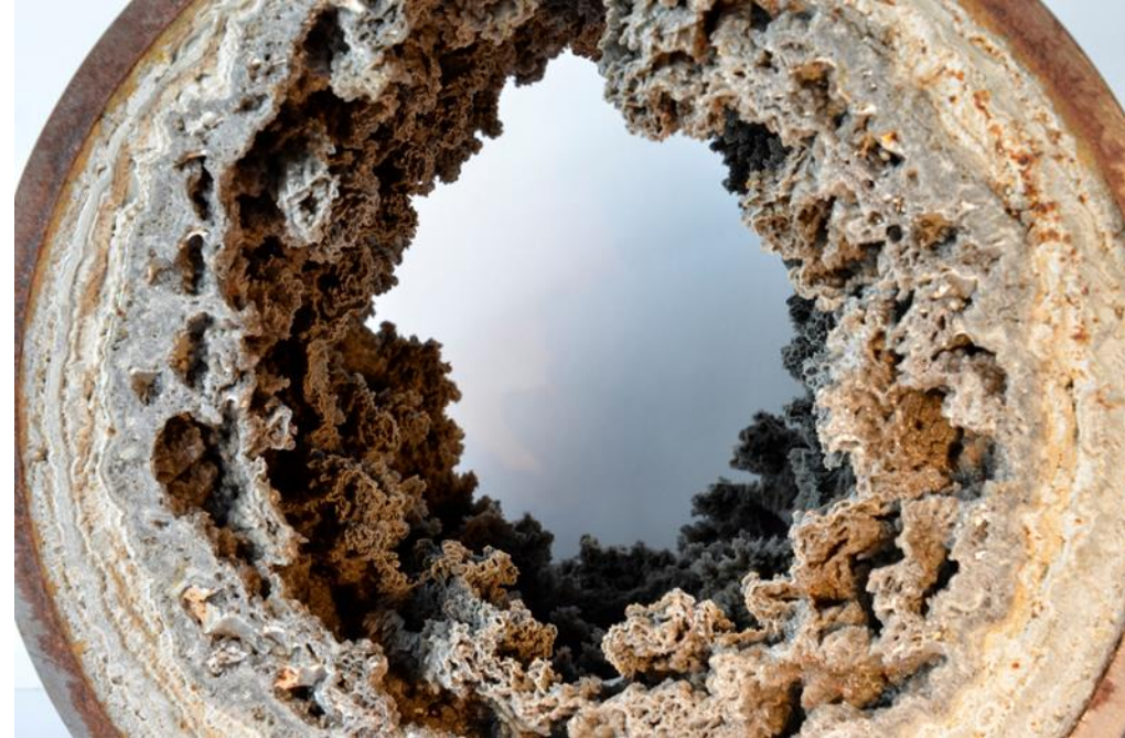
Silica scaling of 450mm reinjection pipe at Ohaaki, New Zealand
