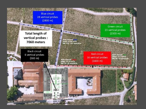
Use of the ground to seasonally balance heating and cooling reducing energy input to the facility Only carbon is associated with the electricity to run the system
