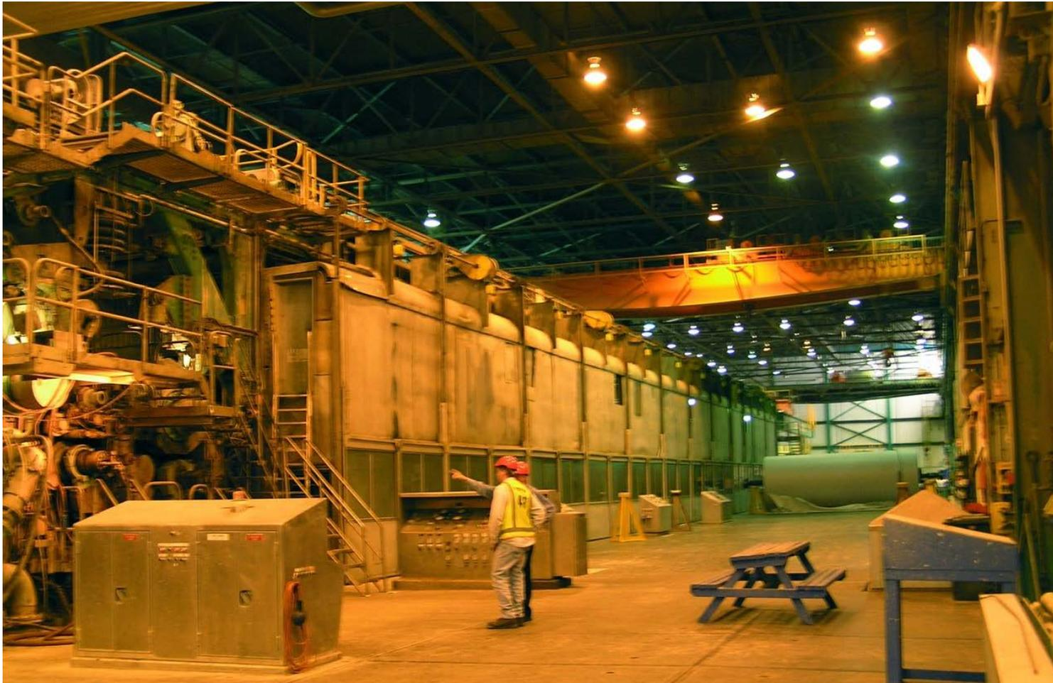
Paper drying at Kawerau using geothermal steam.
