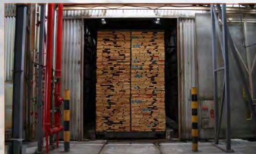
Tenon's timber drying kilns at its Taupo plant use earth energy from low temperature geothermal sources.
