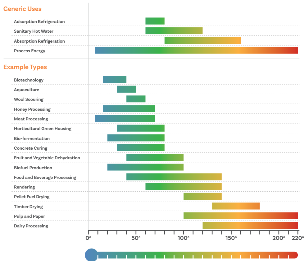
Figure 2 Temperature range for different Geoheat Uses - both Generic and Example types shown
