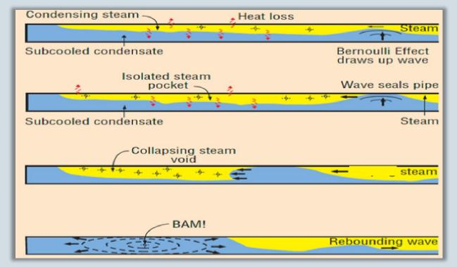
When the steam collapses it generates shock waves which cause a 'hammer' effect that can damage pipework and equipment.
