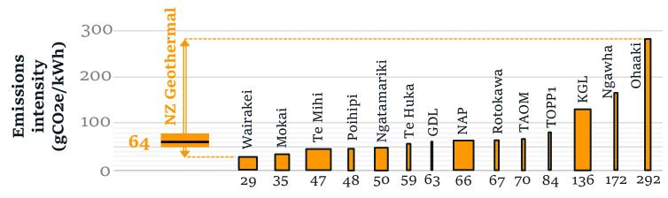
Widths indicate relative plant size, heights are emissions intensity
