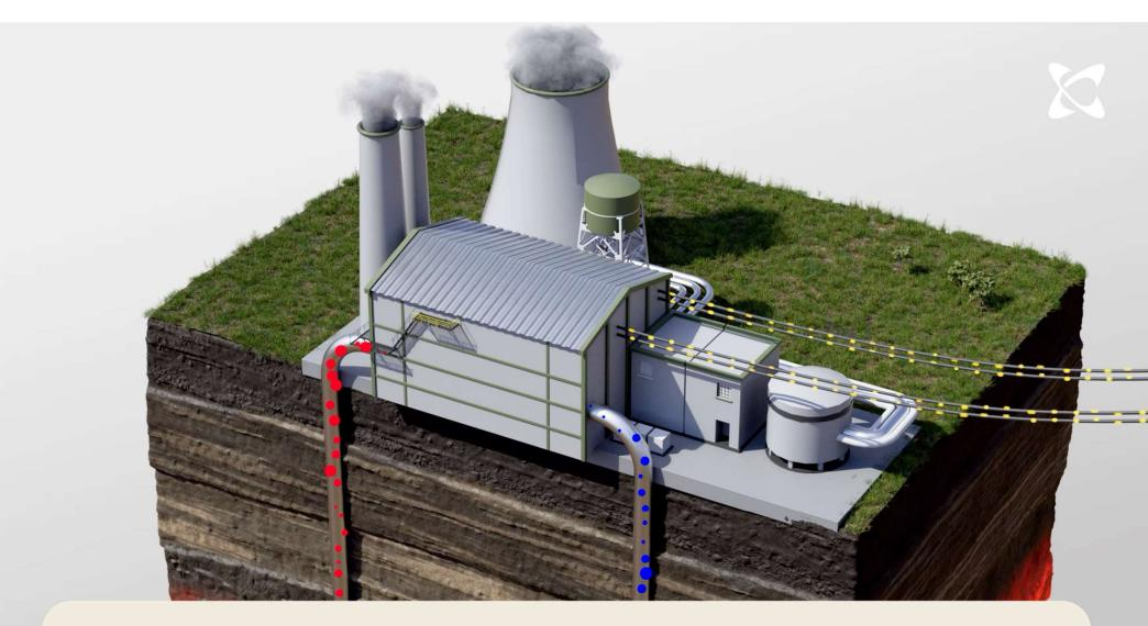
Conversion of heat energy to electricity is only ~10-15% efficient
